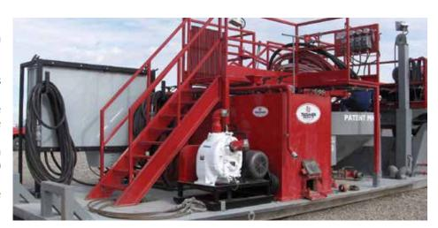
What makes our system so efficient is our patented concentration tank, designed and equipped with a sloped bottom along with a number of cylindrical baffles that circle the inside of the tank from the centre to the outside tank wall.
