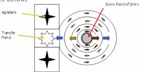
This solids concentrating process blocks most of the fluid in the TecTank from entering the centrifuge(s) through the centrifuge suction. This allows for mainly solids to enter the centrifuge(s), and is essentially what keeps the separation process so efficient.
